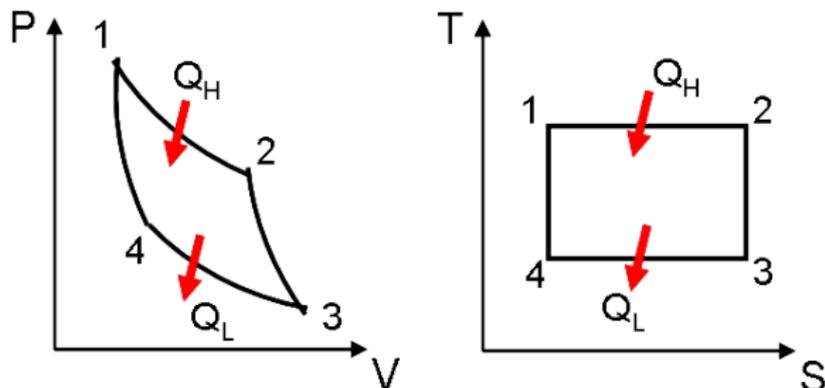
Fig.1. P-V and T-S diagrams of Carnot Cycle
