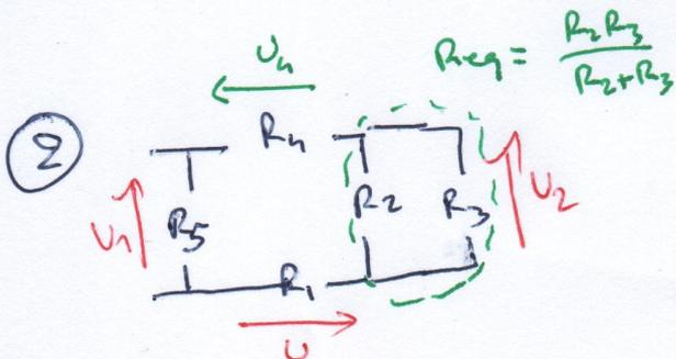
$$\left\{ \begin{aligned} U &= \frac{R_1}{R_{eq} + R_1 + R_4} U_1 \\ U &= -\frac{R_1}{R_1 + R_5 + R_4} U_2 \end{aligned} \right.$$
