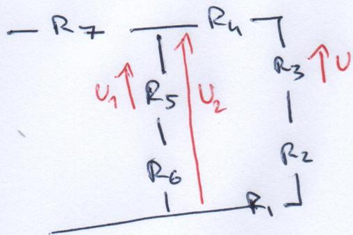
$$\begin{cases} U = \frac{R_3}{R_3 + R_4 + R_2 + R_1} U_2 \\ U_1 = \frac{R_5}{R_5 + R_6} U_2 \end{cases}$$
